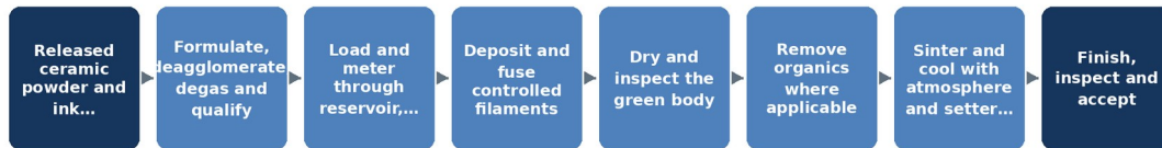
Figure 1. State-resolved ceramic direct-ink-writing route.
