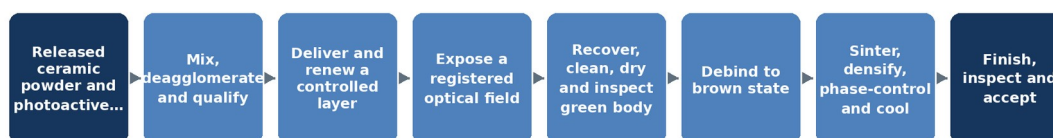
Figure 1. State-resolved ceramic vat-photopolymerisation route.
